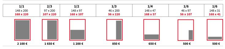
**BLEED formats** are listed in a net format after crop. As for crop, it is needed to make an over-drawing 5 mm from each side.
